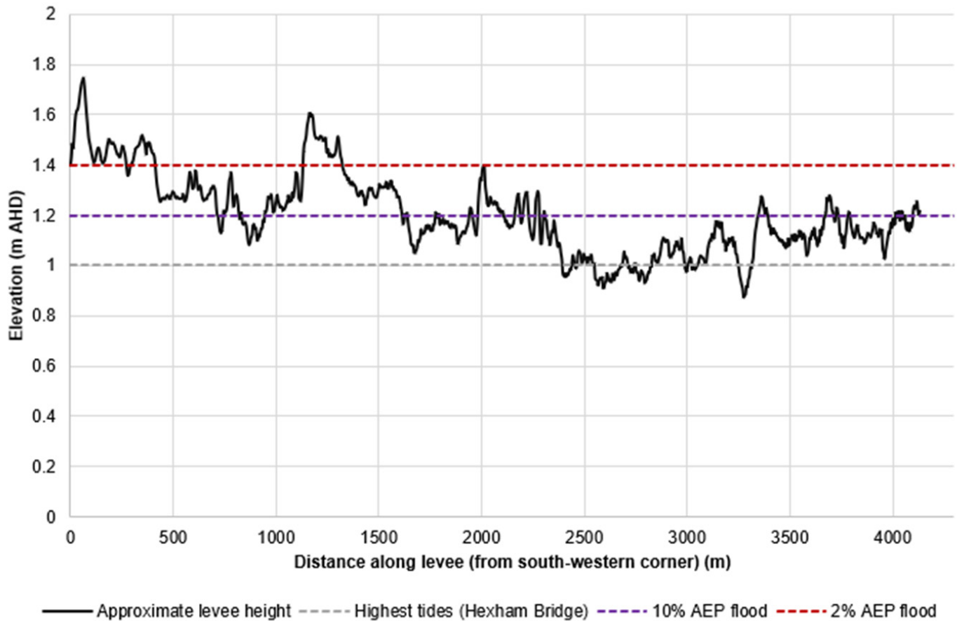
Figure 4.4: Approximate height of the Fullerton Cove levee (derived from GeoScience Australia DEM), compared to flood levels in Fullerton Cove.
