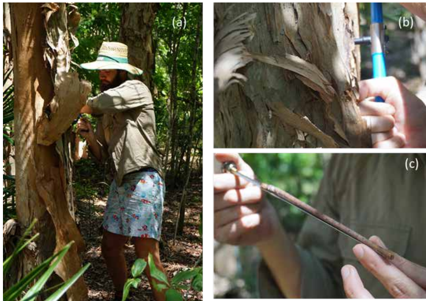
Figure 8.6: Sampling for wood cores from a Melaleuca tree to obtain N and P concentrations, Insulator Ck, Qld. Picture M. F. Adame.
