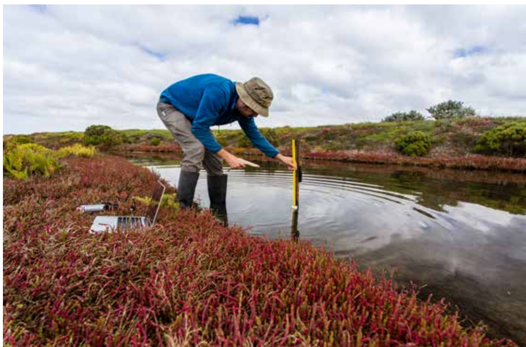
Figure 6.4: Researcher deploying water level loggers, and measuring salinity and pH in a coastal wetland.
