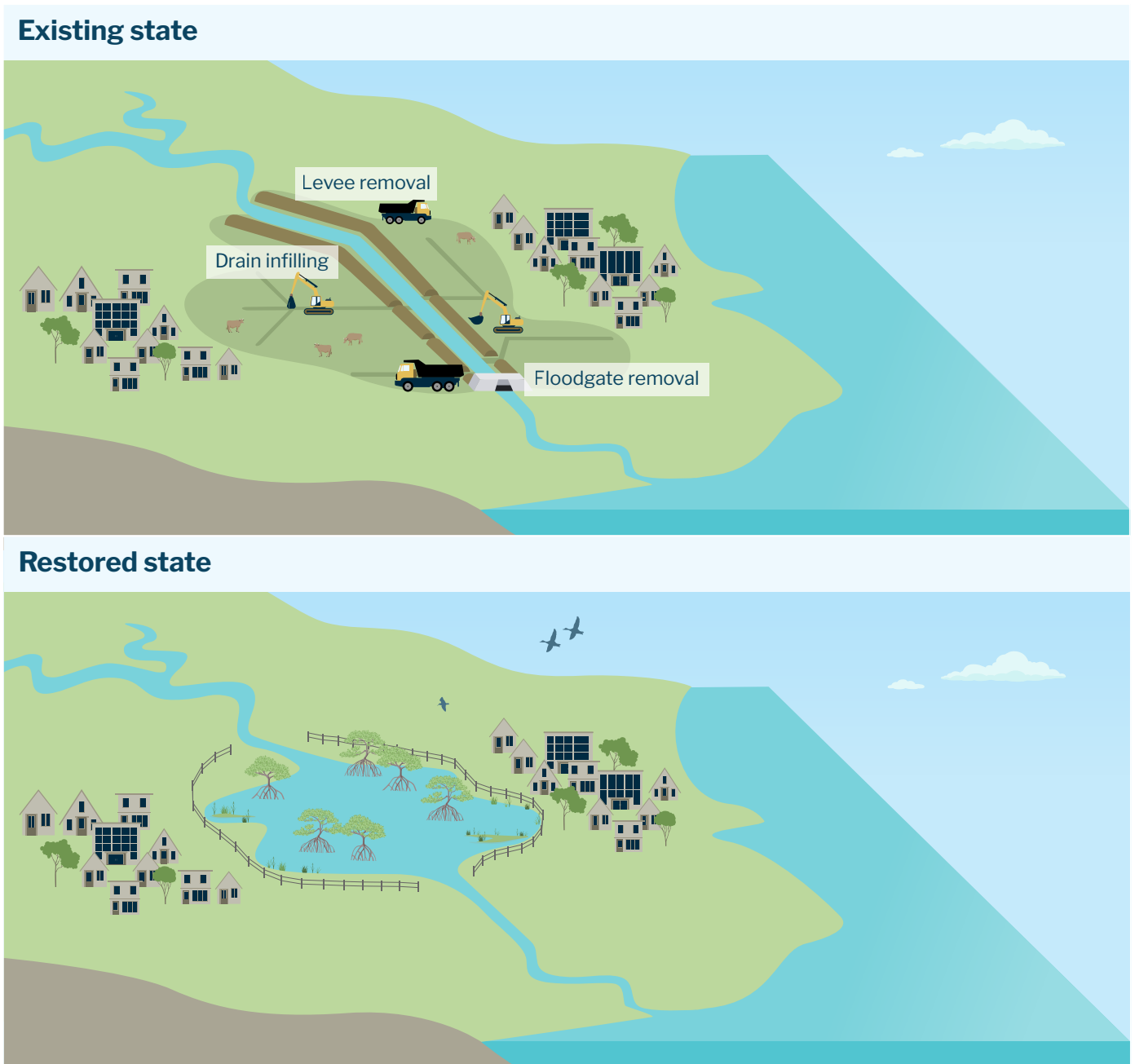
Figure 4.10: Conceptual diagram of restoration activities (such as levee removal or drain infilling).
