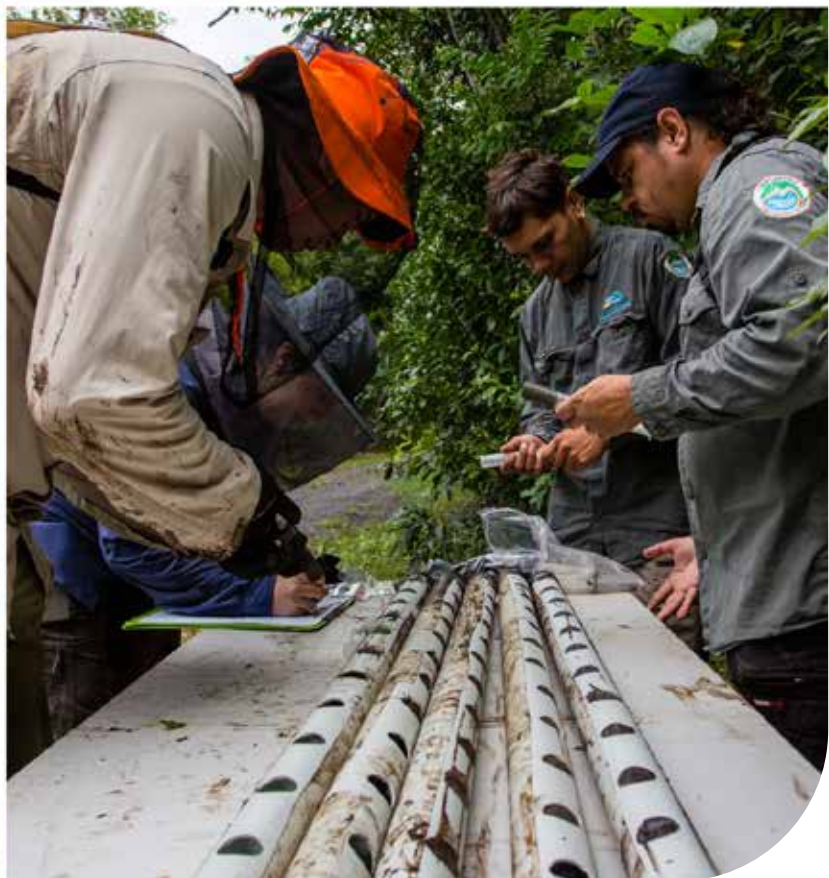
Figure 4: Collection of soil cores in Cairns' mangrove forests with pre-drilled PVC pipes. The sediment sub-samples were collected with use of 30 ml syringe from top, middle and bottom sections of the pre-drilled PVC pipe.
