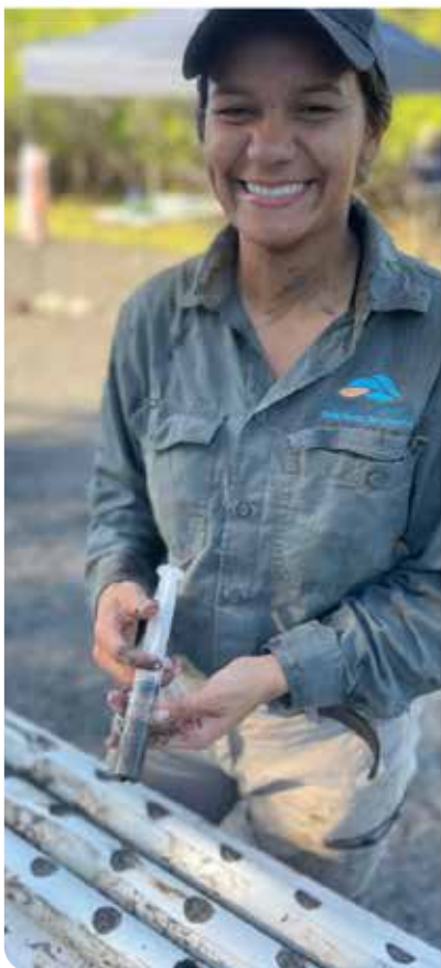
Figure 4: Collection of soil cores in Cairns' mangrove forests with pre-drilled PVC pipes. The sediment sub-samples were collected with use of 30 ml syringe from top, middle and bottom sections of the pre-drilled PVC pipe.
